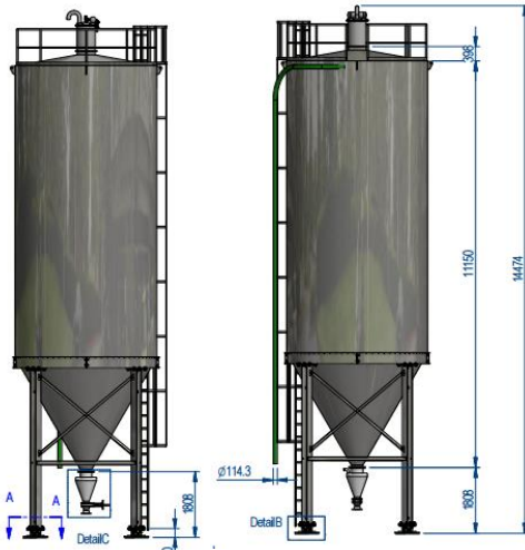
100 m 3 Stainless Steel PVC Resin Storage Silo system
