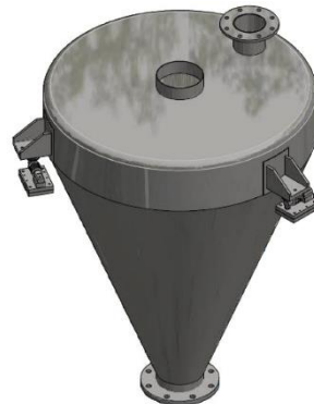
Well Polished , Steep Angle Weighting hopper , with all the bulk material gravity flow assistant component
