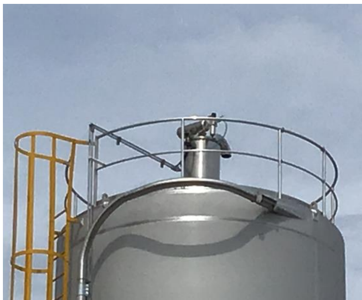
TRC 70.18.500.1000 Compact BF Wheat Flour Silo Vent Application
