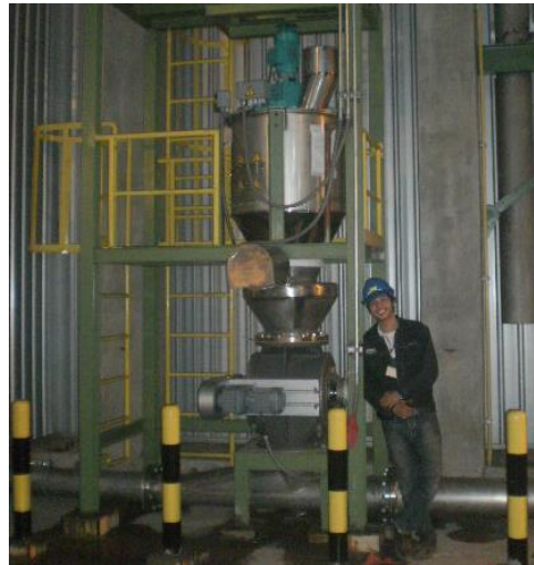
Schenck Accurate Mass Flow Meter set
