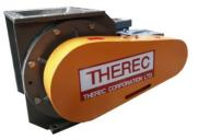
In board bearing pellet handling rotary valve for high vacuum and low pressure pneumatic conveying system Vacuum down to – 500 mBar Pressure up to + 200 mBar Size 6,8,10,12,14,16 inches
