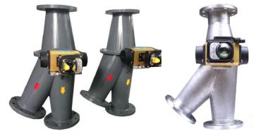
Flap Type, powder & pellet handling diverter valve for medium vacuum & high pressure pneumatic conveying system Vacuum down to -300 mBar Pressure up to + 500 mBar Size 3,4,5,6,8,10 inches
