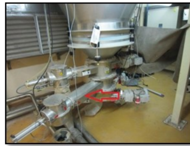
3 screws at 1 feeding point option.
