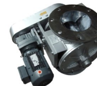
TRC200 Chain drive for Limestone
