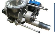
Quick detachable, Easy clean blow through Type, powder handling rotary valve for high vacuum & pressure pneumatic conveying system Vacuum down to -500 mBar Pressure up to + 500 mBar Size 8,10,12 inches
