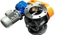
In board bearing powder and pellet handling rotary valve for free flow feeding, high vacuum and low pressure pneumatic conveying system Vacuum down to – 800 mBar Pressure up to + 800 mBar Size 6,8,10,12,14,16 inches
