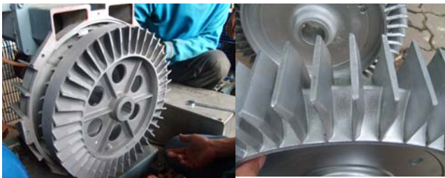
Hard Anodized Coated Surface for The Gas Contact Parts of Cast Aluminium Ring Blower
